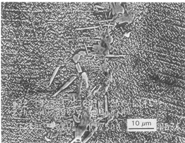
Figure 6 Representative microstructure of the alloy series 72, 73 and 74. Experimental stages consisted of solution at 1378 °C for 2 h, isothermal holding between liquidus and solidus at 1341 °C for 22 h, water quenching and ageing at 900 °C for 600 h. Alloy 72, shown here, exhibits needle-like brittle \eta -phase and carbides which were formed along grain boundaries.
